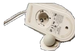
A roller ball mouse requires frequent cleaning.
